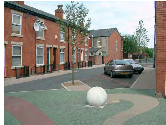
Figure 5.13: Paving can be used to help delineate areas for different activities in a street
