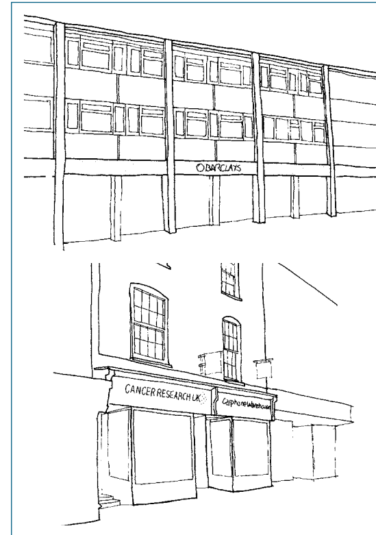
Figure 7.27: In these examples the fascia is in proportion with other elements of the building and fits in with the overall street scene
