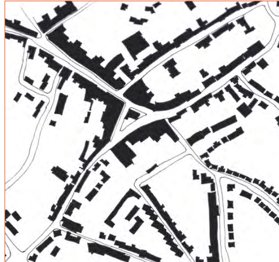
Figure 3B.4: The figure ground of Wokingham Town Centre demonstrates how the built form gives the streets a tightly defined and enclosed character
