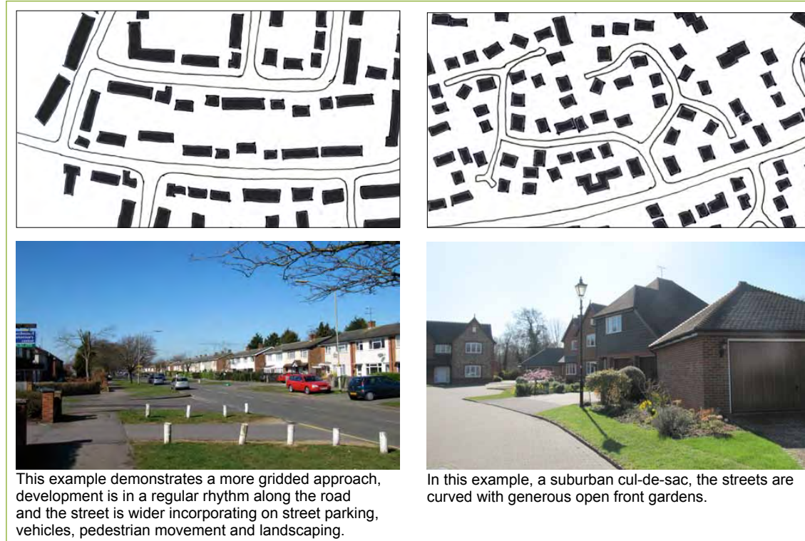
Figure 5.3: Depending on the settlement pattern, streets will have different characters and functions
